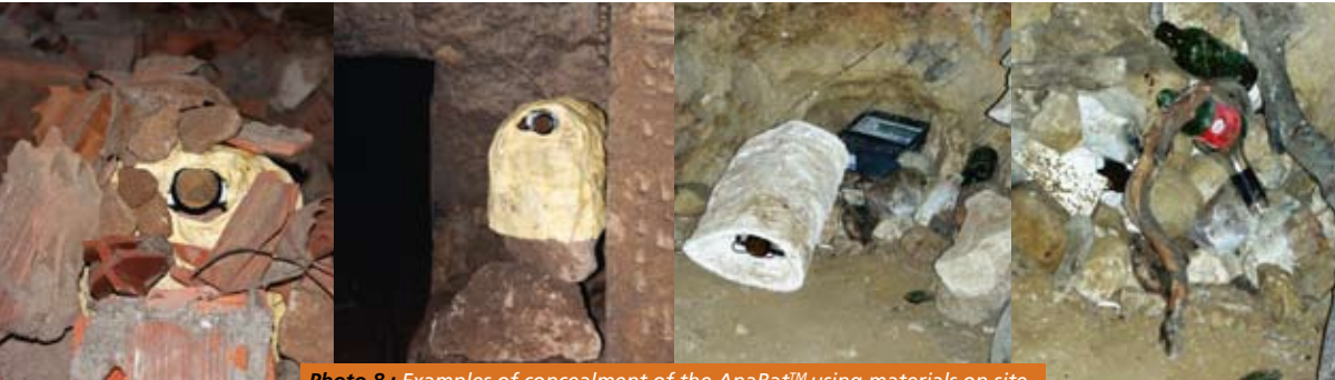
Photo 8 : Examples of concealment of the AnaBat™ using materials on site.
